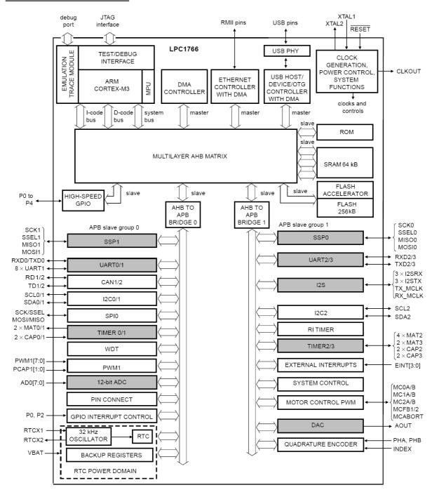
Grey-shaded blocks represent peripherals with connection to the GPDMA.
