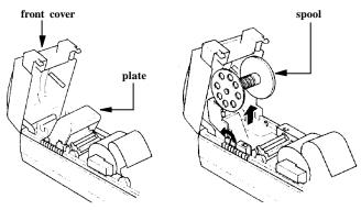
Place the paper roll in and raise the lever as shown in the illustration and place the
