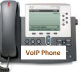
VoIP telephones use the internet to link and are rapidly increasing in usage, overtaking the traditional telephone network. The VoIP system enables notification of calls via email or text.
