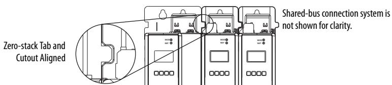
Mount the Kinetix 5700 drive module to the cabinet subpanel with M5 (#10-32) steel bolts torqued to 4.0 N•m (35.4 lb•in), max.
