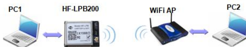
Figure 26. STA Interface Debug Connection
