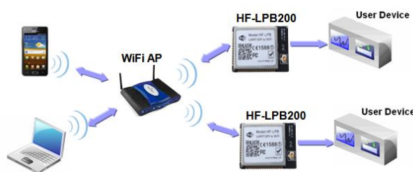
Figure 11. HF-LPB200 Basic Wireless Network Structure
