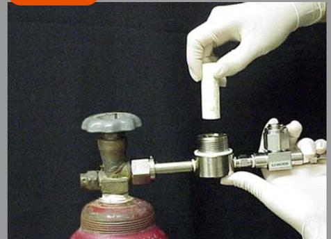
Position LCO<sub>2</sub> Filter Element (#8784A) into center of lower Oil/Water Filter Housing.
