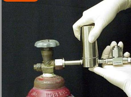
After all of the pressure is safely bled from high pressure line, unscrew Oil/Water Filter Housing by hand.
