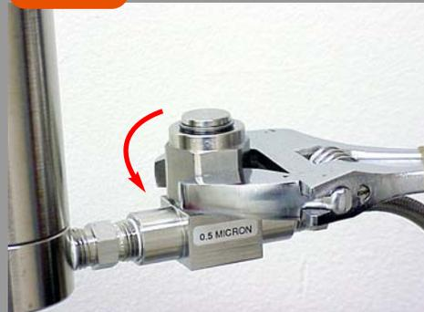
After all of the pressure is safely bled from high pressure line, unscrew T-Filter cap using wrench.
