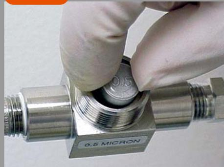
Carefully remove T-filter element.
