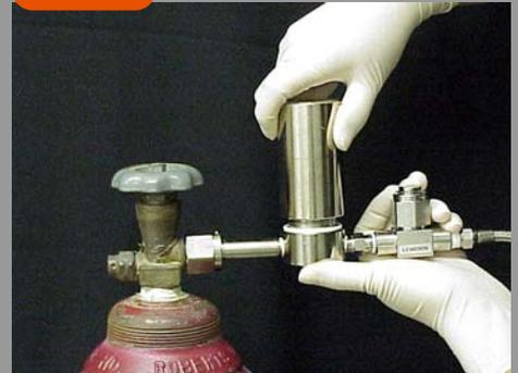
Hand tighten the housing body together firmly. O-Ring seats properly. Open main tank valve and check for leaks.
