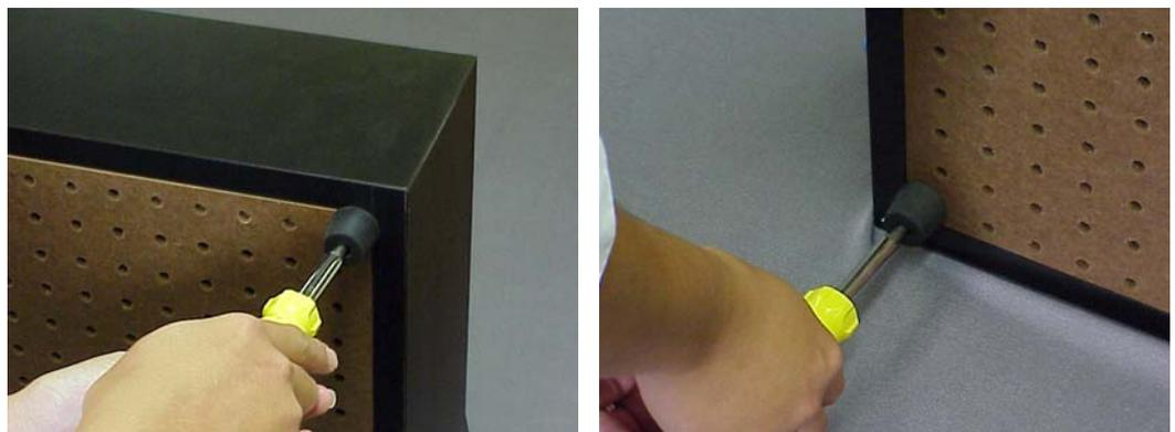
7. Remove and set aside the access panel. Note access panel orientation so that you may re-install panel in the same direction upon procedure completion.
