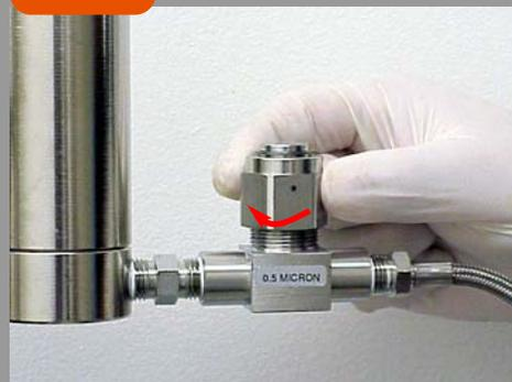
Hand tighten T-filter cap.
