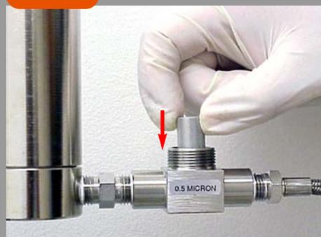
Install a new T-filter element (#8770-83B) into center of T-filter housing.
