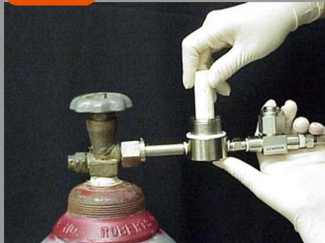
Place new LCO<sub>2</sub> Filter Element (#8784A) into lower Oil/Water Filter Housing. Let gravity hold element in place.
