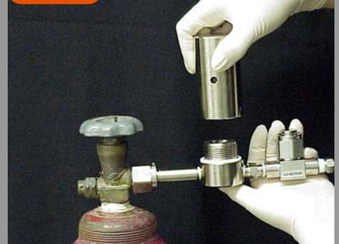
Remove Oil/Water Filter Housing.
