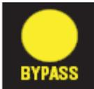
Push once to force the shut-off valve open; push again to return to normal operation. **Caution:** Unit will not shut off water, but will send alarm fault when cap loss is detected.
