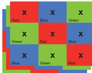
**Colour Light Output** uses 3 sets of a nine-point grid to measure the primary colours - red, green and blue, using the same approach used to measure White Light Output in lumens.
