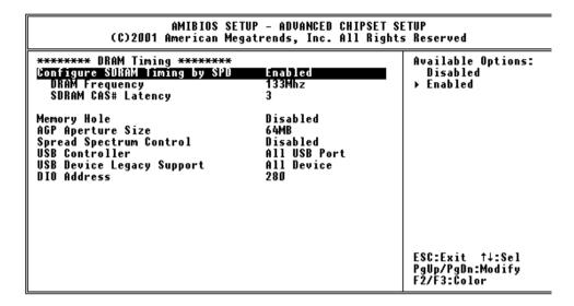
This section enables you to configure the system based on the specific features of the installed chipset. This chipset manages bus speeds and access to system memory resources, such as DRAM and the external cache. It also coordinates communications between the conventional ISA bus and the PCI bus. It must be stated that these items should never need to be altered. The default settings have been chosen because they provide the best operating conditions for your system.
