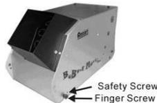
To help avoid accidental exposure to dangerous live AC main voltage, two safety screws are fitted that require a screwdriver to remove. Once these are removed, the finger screws can be undone by hand (see photo above).
