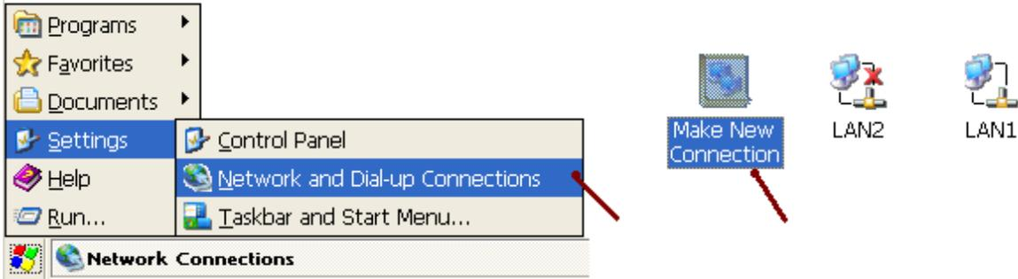
Select “Dial-Up Connection” and type an English name (ex. GPRS, it allows to contain the numbers 0 to 9) then click “Next” and select the modem - “ICPDAS I-821xW MSA1:” .
