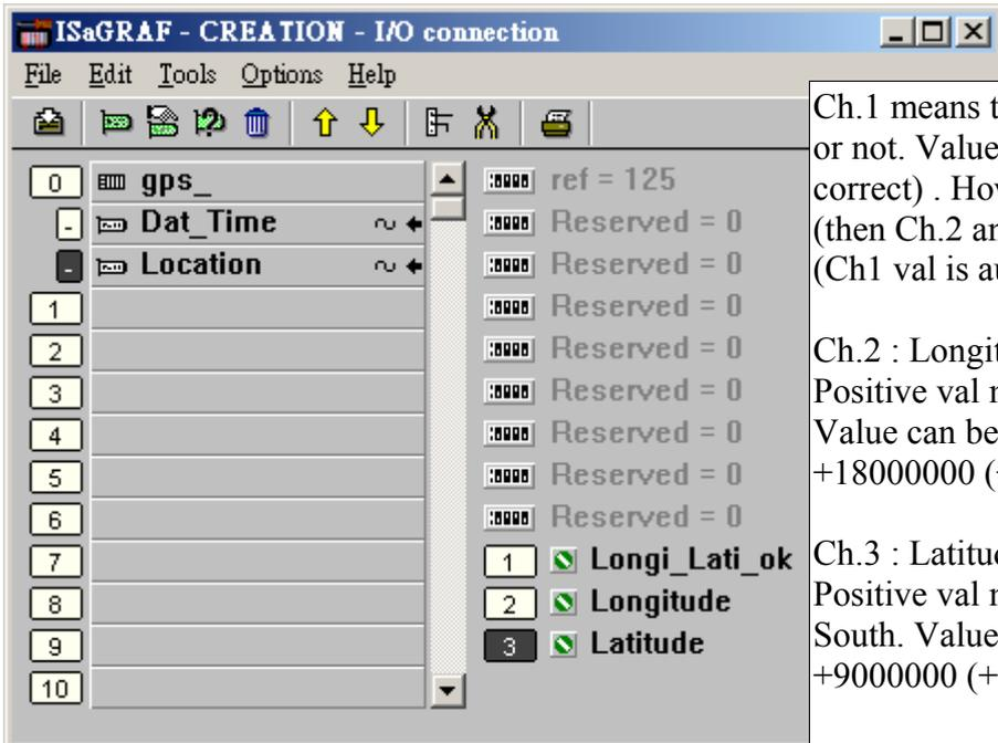
Ch.1 means the Longitude and Latitude correct or not. Value 1 means correct (Ch.2 and 3 are correct) . However value 0 means incorrect (then Ch.2 and 3 data can not be used) (Ch1 val is auto-modified by the satellite state)
