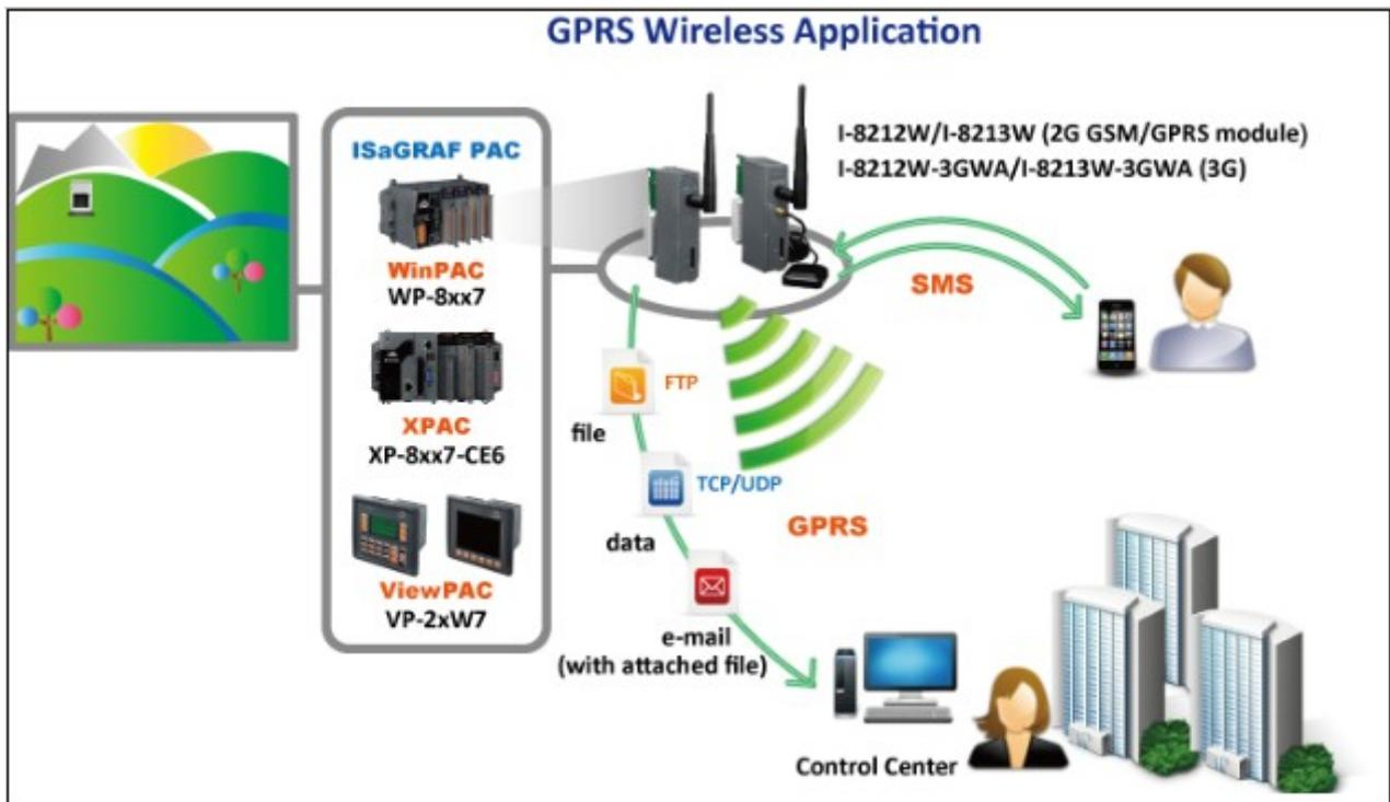
The following ISaGRAF driver version supports the dial-up GPRS (2G) access with I-8212W .
