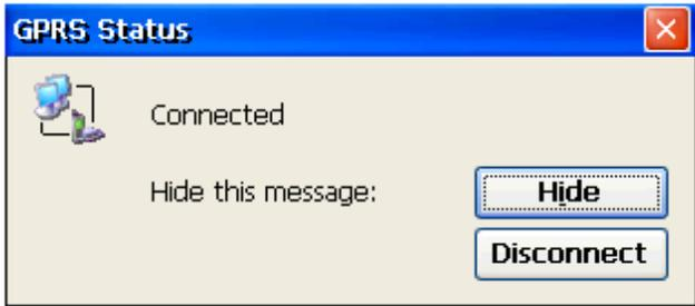
After successfully connecting, open "Command Prompt" and give a ping command to check if the connection is fine (If ping internet fail, refer to the next section 1.2.3 ). After ping is ok, must run "Disconnect", then continue the next important steps .
