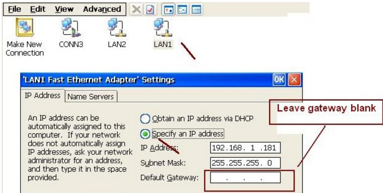
If your PAC can connect to the Internet by using LAN1 or LAN2, then recommend not to use the GPRS (in such a case, then please set the gateway of LAN1 or LAN2). The reason is LAN1 / LAN2 speed is much faster than the GPRS.
