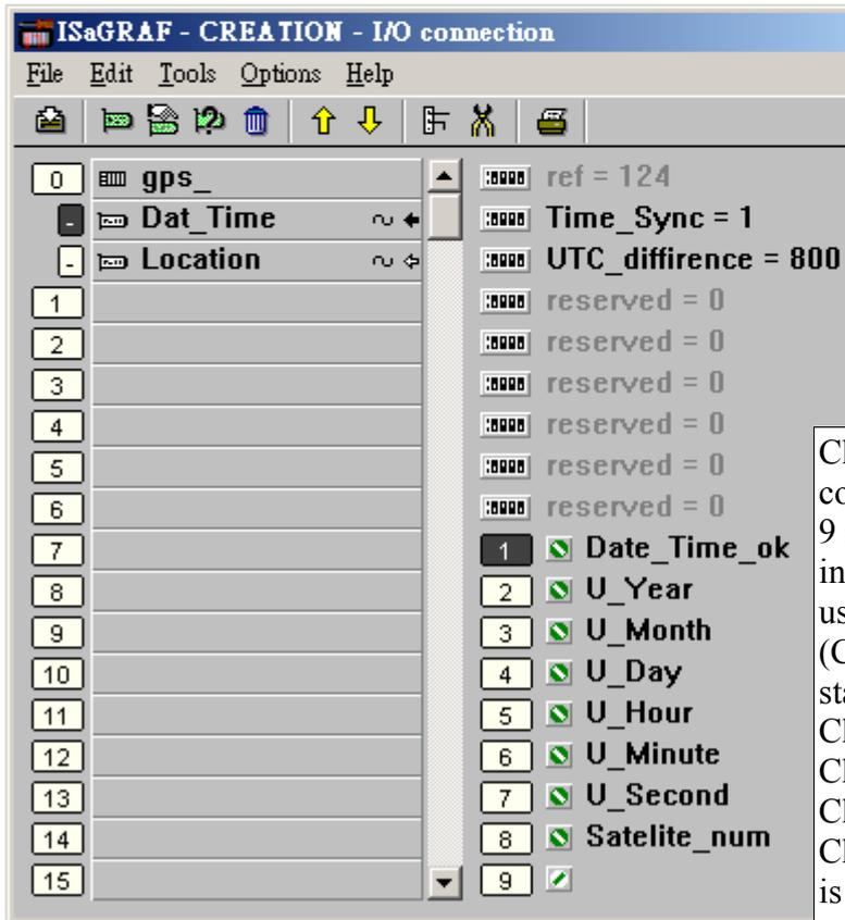
Time\_Sync: value 1 means enable the auto-time-synchronization function. Value 0 disable it.
