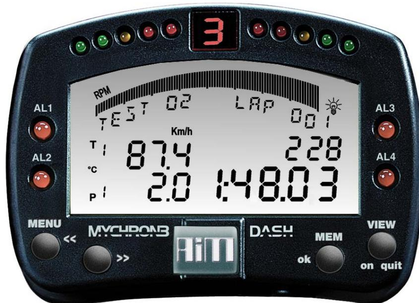
When the session is over it is possible to recall stored data pressing “MEM/OK”. The display shows, under the RPM Bar graph, test and lap number the data showed in the other fields refer to: in the above image: “TEST 02 – LAP 001”.
