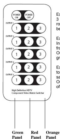
Example 1 – You would like to route your DVD player on Input 3 to Output 1. Press the number 3 button on the Output 1 row. The LED of Output 1 on the front panel of the switch will be illuminated orange.
