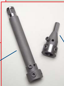
3/4" Weldon Shank (2 Flats) 6" length (p/n 7-9-906) 12" length (p/n 7-9-912)
