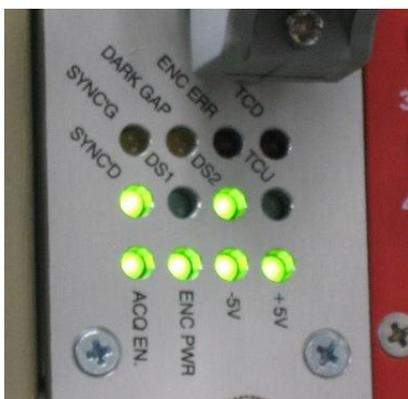
LED indicators on the Chopper Controller in the NIM Crate show the status of the chopper system.
