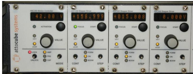
The ANC350 front panel is shown above. The first slot is the master module, and shows the driving voltage of the module in focus. The second and third modules are for the Analyzer and ATH motors, respectively. The current angular position or holding voltage is shown. Refer to Attocube User Manual for more information.
