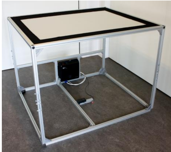
Figure 11.1c. This is the setup for the multitouch table. The acrylic glass includes Orgasol spreading the lights evenly. To break the bouncing of infrared lights in the glass, a compliant layer of silicone and Xylol is added to its surface. The camera is a Logitech 9000 with a wide angle and a high resolution.
