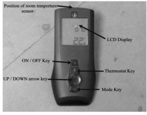
c. With the appliance lit, by pressing key the operational mode is switched from manual to Room thermostat setting and vice versa. When Room thermostat mode is active, the display shows the
