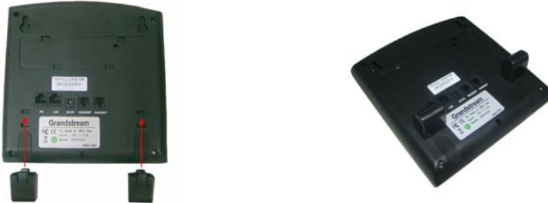
Figure 2: Attach the wall mount spacers to the GXP1200
