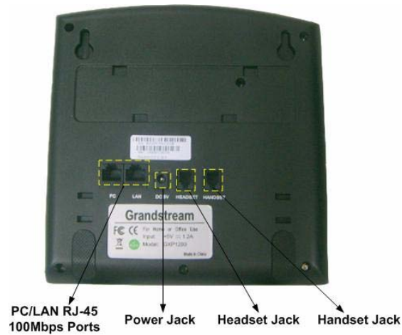
Figure 1: Connectors on the bottom of the GXP1200
