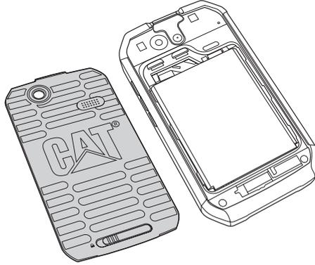
2. Engage the hooks on the top of the back cover with the designated holes on your phone.
