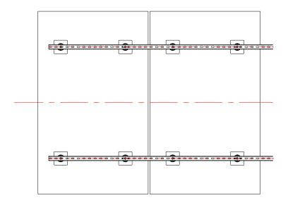
Fig.3 Two double glass modules are mounted on the brackets.
