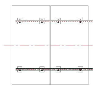
Fig. 7 Two 72 cell modules are mounted on two brackets
