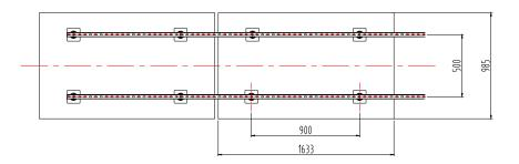
Fig. 5 Two modules are mounted along the long edge
