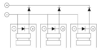
(2) The bypass diode should have a Rated Average Forward Current at least 10A, and a Rated Repetitive Peak Reverse Voltage of
