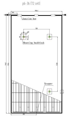
Fig. 6 The array of backblocks on 72 cells double glass modules
