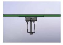
Fig.4 Backblocks fastened on U-shape brackets by bolt
