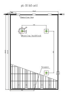
Fig.1 Array of backblocks on the module
