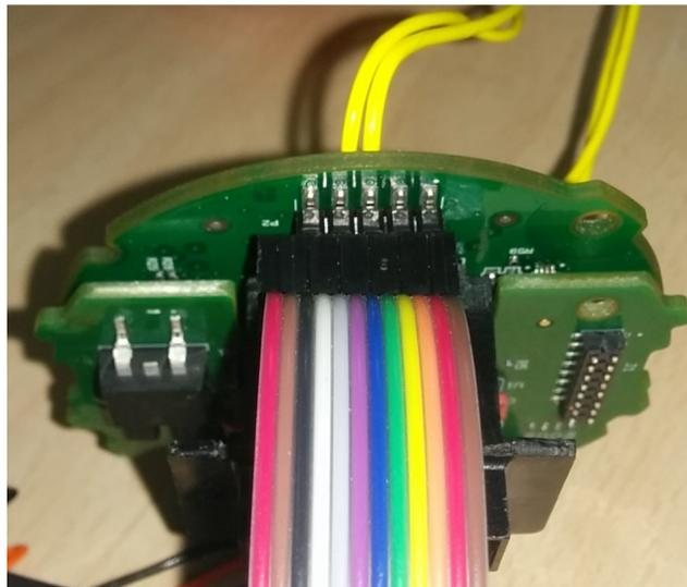
**Figure 1: Level transmitters only - Ribbon Cable Assembly and Fieldbus board**
