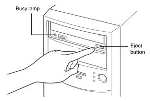
2 With the label side of the CD facing upward, put the CD in the center of the tray.
