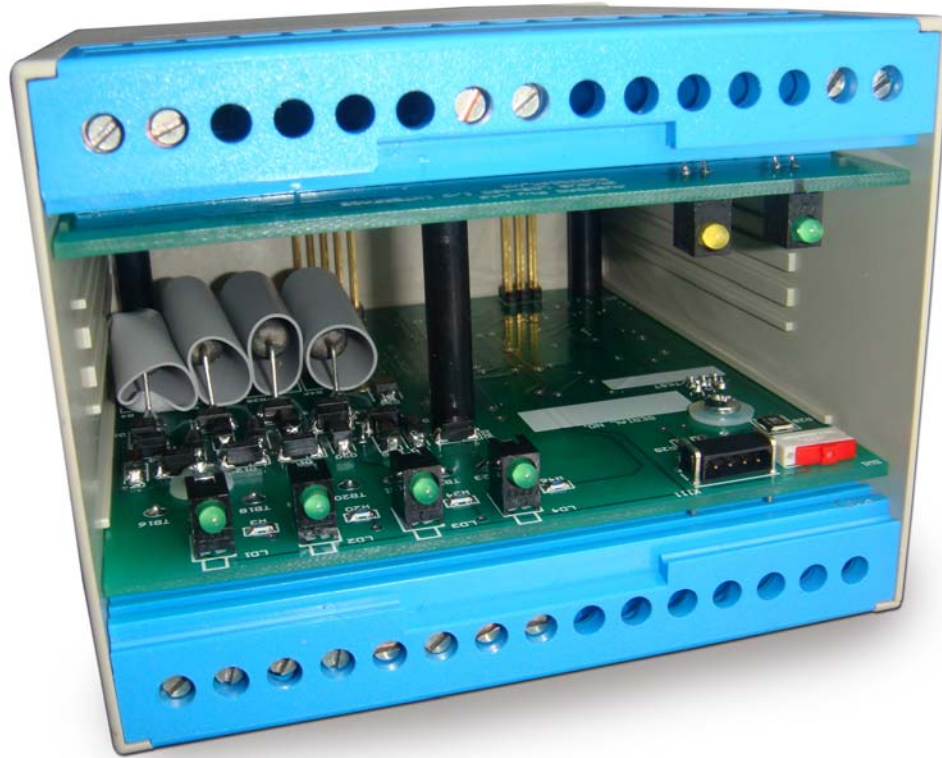
Photograph 2 Access to console port and programming switch
