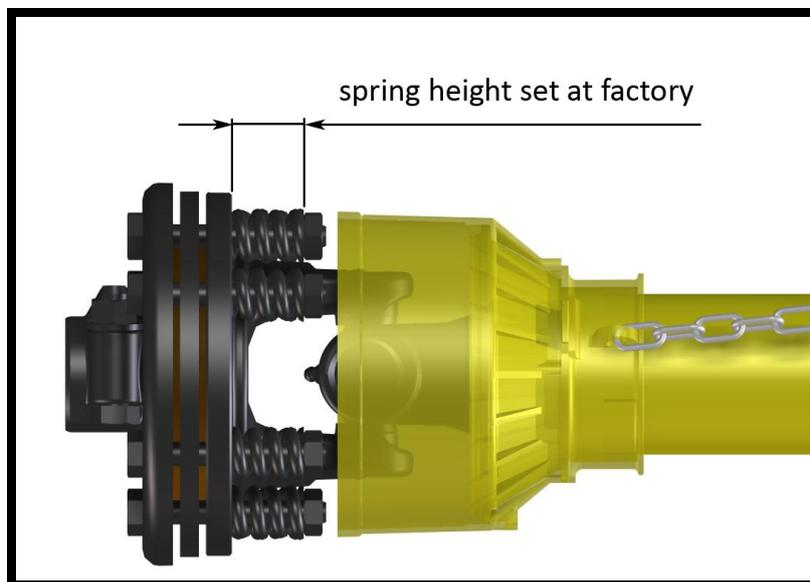
An adjustment can be done, however, when the clutch slipping is too frequent, which means that the calibration is too low.
