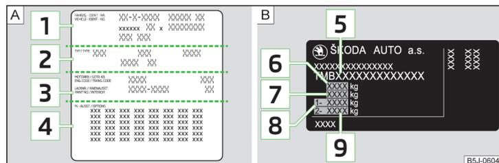
Fig. 212 Vehicle data sticker/type plate
