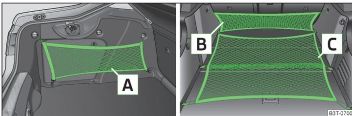
Fig. 100 Fastening examples for nets
