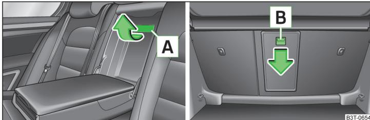
Fig. 97 **Rear seats: Cover handle/boot: Unlock button**
