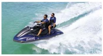
**Planing** is a faster speed where the bow and the stern of the PWC are level. The entire craft is skimming on top of the water, which creates a minimal wake.
