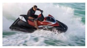
This connection between steerage and power is the most critical aspect to understand about operating a PWC and cannot be over-emphasised. Many accidents have occurred when a PWC operator has collided with objects or people after turning off the engine or reducing power.
