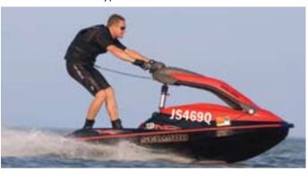
**Performance-orientated PWC (stand-up):** Featuring a hinged, adjustable steering column, the rider stands or kneels on a platform at the stern of the boat. These are often used for racing, and require skill and balance to operate. They can accommodate only one rider.
