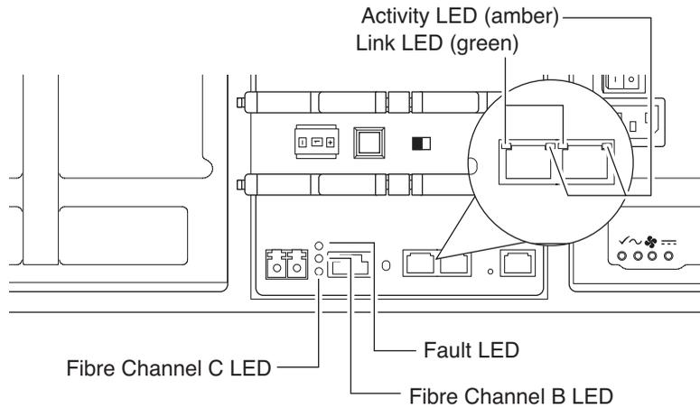
**Interpreting Ethernet LEDs on a FAS270/FAS270c:** Use the following table to interpret the Ethernet port LEDs on the FAS270/FAS270c CPU module.
