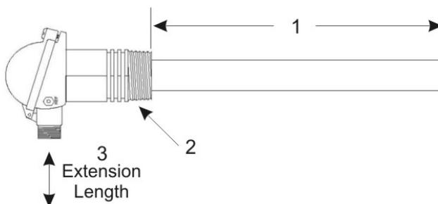
*Figure 2-2: Model 9060L Probe*
