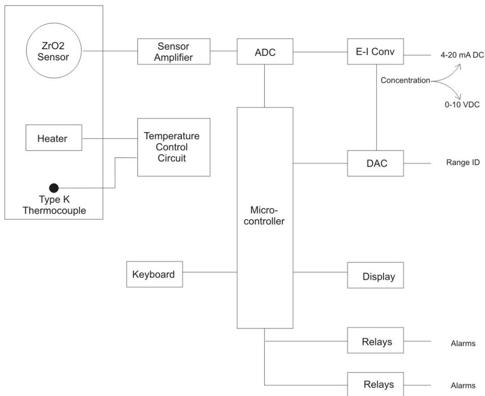
Figure 2-3: Signal Processing Block Diagram
