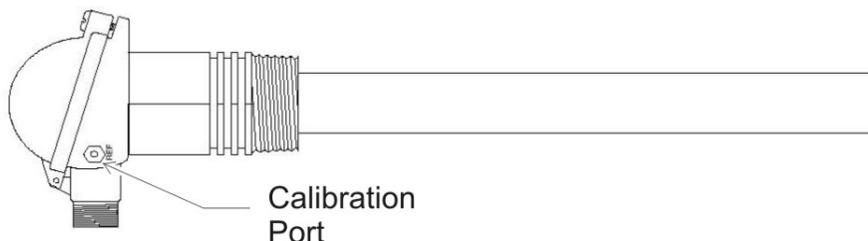
Figure 4-2: Calibration Port on Probe Head
