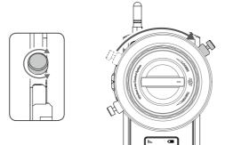
2. The travel range of the focus wheel is now limited to the distance between the two hard stop screws.
