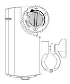
The motor can be clamped to a 15 or 19 mm support rod. To clamp the motor to a 19 mm support rode, first remove the two adapters on the clamp:
