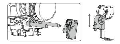
Tighten the knob to secure its position. Ensure the motor gear and lens gear ring make good contact. Ensure the lens gears are not too tight to avoid premature wear to the gears or damage to the lens.
