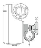
2. Push the knob away from the clamp and open up the clamp. Slide and remove the two adapters on the clamp.
