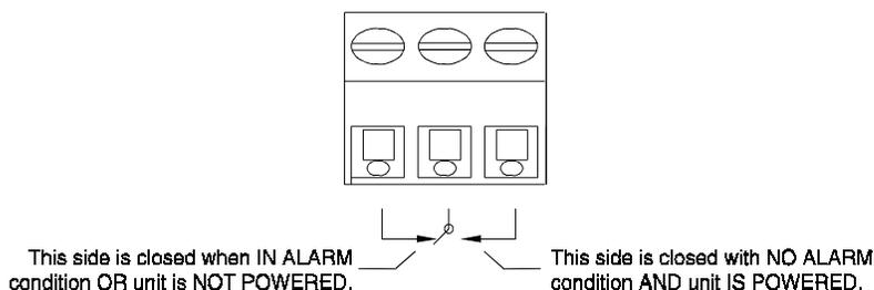
Figure 3-2: Contact ID for FAILSAFE Relay Operation
