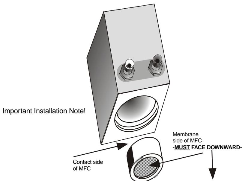
During the Installation and/or Replacement of the MFC, **Membrane** surface **MUST ALWAYS FACE DOWNWARD**, and the Contact side of the Membrane, **MUST** be placed **FIRST** into Analysis Unit.
