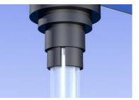
clockwise about one turn until the tissue surface is in focus. Turn a little more to focus on the capillaries below the surface.
