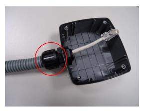
8. Tighten the domed sealing nut.
