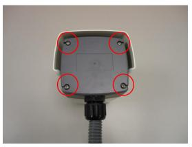
10. Tighten the screws of the back side of the camera properly.
