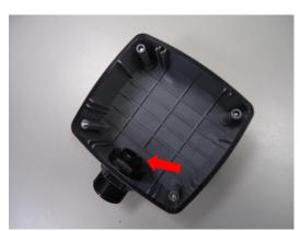
5. The fourth piece (locking nut) is used to lock the gland firmly from the inside of the back side cover.
