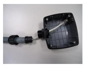
6. Pull the network cable through the back side cover of the camera.
