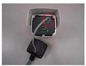
9. Plug the network cable into the camera's RJ-45 connector before closing the back side of the camera. If you are not using PoE and need an additional power cord then please connect it at this stage, too.
