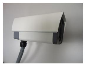
11. Finally, the box camera with properly mounted flex conduit as well as with proper outdoor bracket would look like this.
