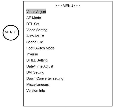
2. Select an item by Arrow Keys ♥ on the front panel of CCU, and press SET switch to define the mode.
