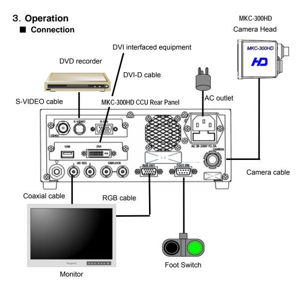
\* Terminate the output from RGB OUT and VIDEO OUT at 75ohms on the receiver side.
