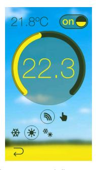
By clicking on this icon, a control dialogue appears and allows to switch on/off the thermostat or setting a new set point temperature by sliding the finger over the circular scroll bar (the command is sent when release). The current measured temperature is also indicated at upper left corner (from 0 to  $51\,^{\circ}$ C).
