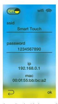
The Wi-Fi network is generated by the Smart Touch with the name (SSID) and password configured in this menu. This network has no internet access, so it is not possible to navigate through the web or control the home automation system from outside the house or installation.
