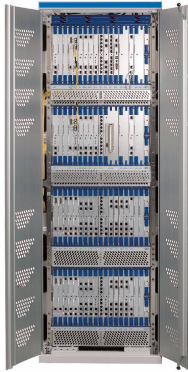
Figure 3-3: An IPA2800 based one cabinet network element [10]
