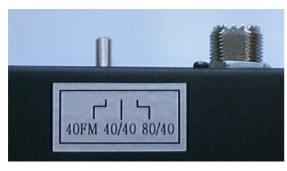
Before You install Your new CB radio, You should preset the country switch on the rear side of the radio according to the local authority requirements. Because this radio is used in most cases by truck drivers in central and western Europe, it comes programmed with the center switch position 40/40 channels. If You are in a country where this setting should not be allowed,
