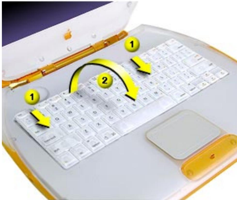
5. Press down on the two keyboard release tabs (located on the keyboard between the F1 and F9 keys), and slide them toward you.
