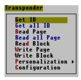
Get ID: Reads the ID number of the transponder located in the field of the antenna.
