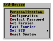
**Personalization:** Submenu to change keys and passwords of the read/write device.
