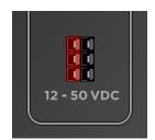
To charge your unit, insert the DC charging cord that is connected to your charging source (solar panel, hand crank, windmill etc.). The LCD display will show DC:IN, charge level and remaining charge time. Once the unit is fully charged, the display will read FU:LL (Please note: When the unit is close to fully charged, the display will flash and read 00:01 for 5 to 20 minutes until the cells in the unit are balanced and fully charged)
