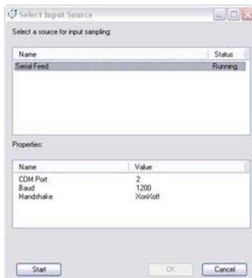
The Select Input Source window; in this case only a single source is available for selection
