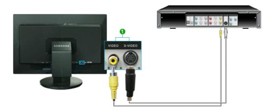
Input devices such as DVD, VCR or Camcorder are connected to the RCA or S-VIDEO terminal of the monitor using the RCA or S-Video cable.
