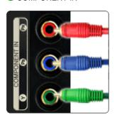
Connect the VIDEO OUT port of the DVD / DTV Set-Top Box to the Y, PB,PR input ports using a component video cable (Y, PB,PR).
