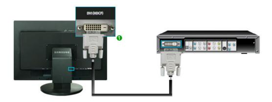
Input devices such as digital DVD are connected to the DVI IN terminal of the monitor using the DVI cable.
