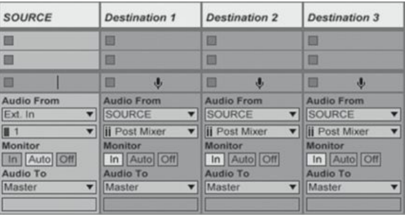
Figure 6.8 The three “destination” audio tracks are all receiving the signal from the track called SOURCE.
