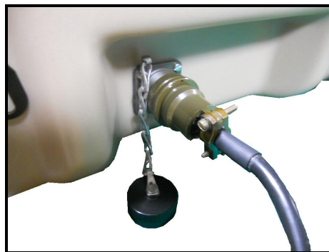
Thread outer shell onto connector until hand tight
