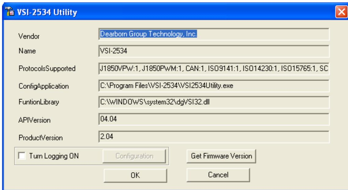
**Protocols Supported:** J1850VPW, J1850PWM, CAN, ISO9141, ISO14230, ISO15765, SCI\_A\_ENGINE:1, SCI\_A\_TRANS:1, SCI\_B\_ENGINE:1, SCI\_B\_TRANS:1, SWCAN\_ISO15765\_PS, SWCAN\_PS, GM\_UART\_PS
