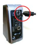
**Step 3.** Connect the square end of the USB cable to the hard drive. Then connect the flat end of the USB cable to the USB port on your computer.
