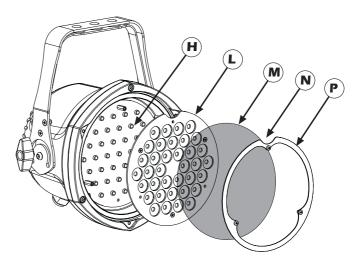
To further increase the beam angle the "R" flood reflector is available (code **CO9168**) and it must be fitted instead of the lenses group and filter holder. For the user of IR remote control: ensure that the "N" slot is aligned on the reflector where the IR sensor is located on the side of led disc "H".
