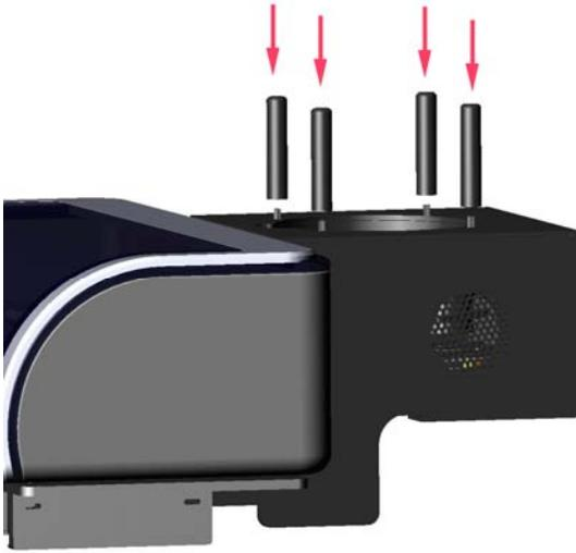
**Fig. 2** Mounting the input holders
