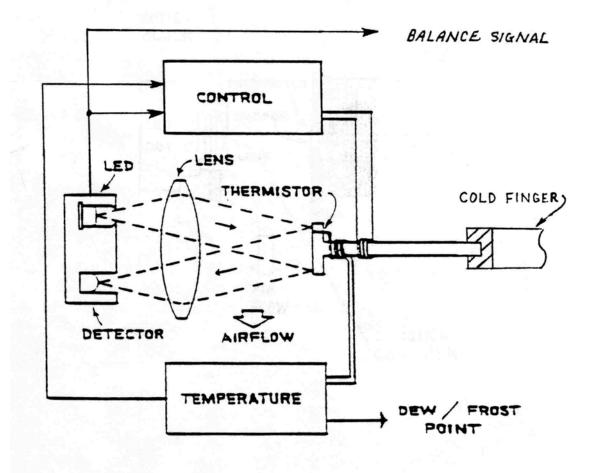
Fig. 2. Block diagram, CR-1A chilled mirror hygrometer
