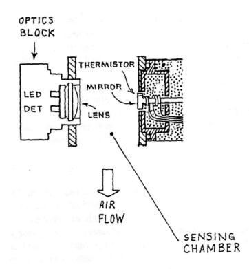
Fig. 3. Sensor assembly block diagram
