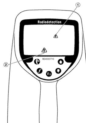
If there are more than 30 volts on the line the second HI VOLTS symbol (number 2 on illustration) flashes on and off.
