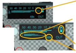
In "multí" mode three additional bars show the 3 input channels post-fader levels.
