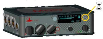
Hold down the ESC button for >2 seconds to turn MIXY off.
