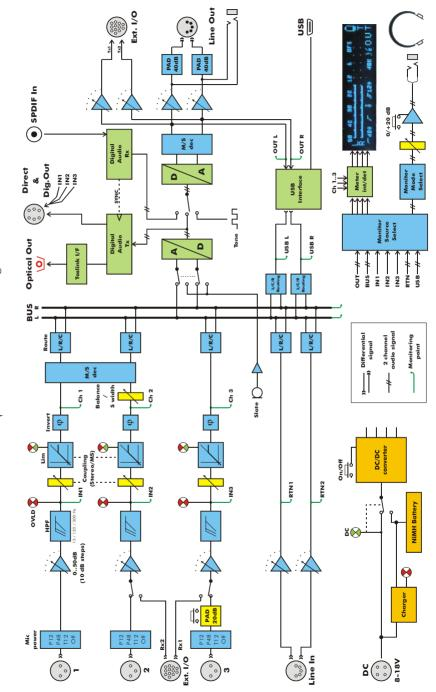
MIXY block schematic diagram
